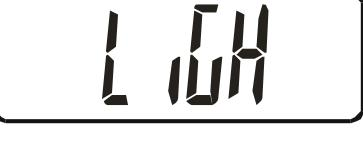
. *『onoff- means auto-backlight, off- means backlight off, ON- means backlight on』*
